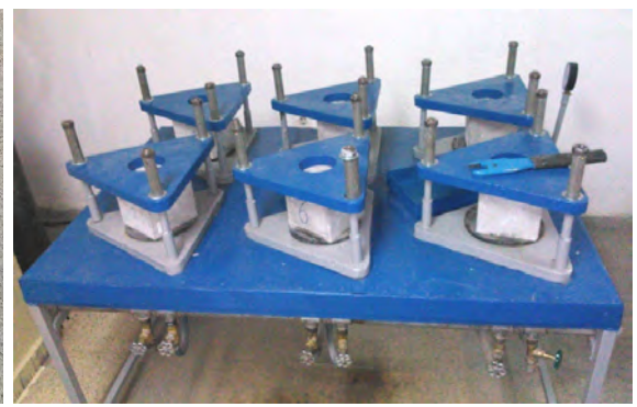
* Testing the resistance of concrete to water penetration under pressure
