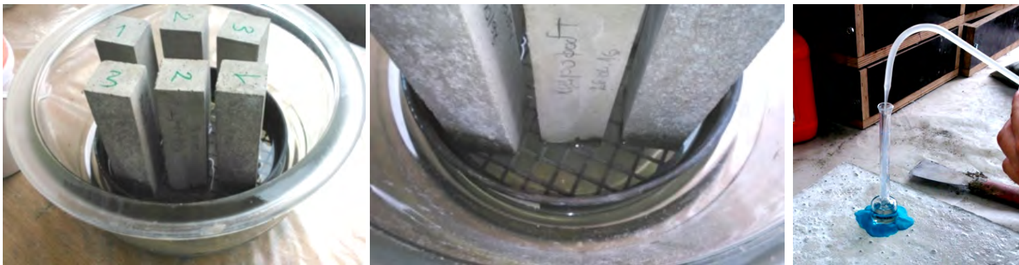
* Testing of concrete resistance to capillary absorption
