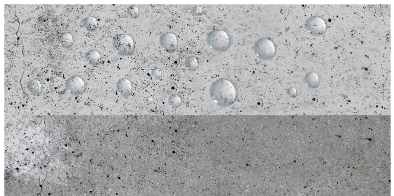
*Water-repellent concrete surface
