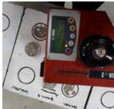
Examination of the adhesion of protective coatings Pull – off method
