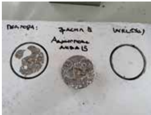
Examination of the adhesion of protective coatings Pull – off method
