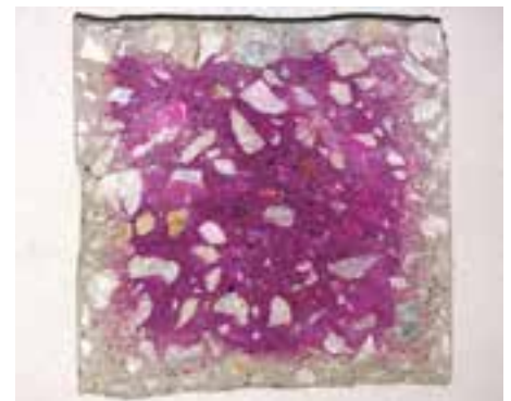
Examination of depth of carbonation
